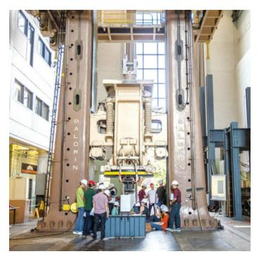
As part of their Structural Behavior Laboratory course, Lehigh University students tested this 10-foot-high concrete column in the 5,000,000-pound universal testing machine in Fritz Engineering Laboratory. The ability to conduct such full-scale testing in an academic setting is a uniquely Lehigh experience.
